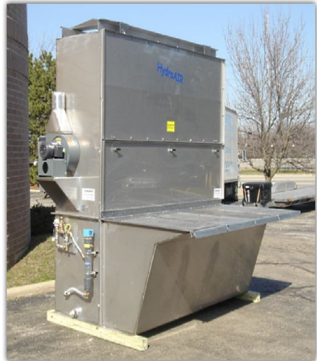
Above: HydroAIR Table Unit equipped with "Magnesium 24-7 Powered Off-line" ventilation
