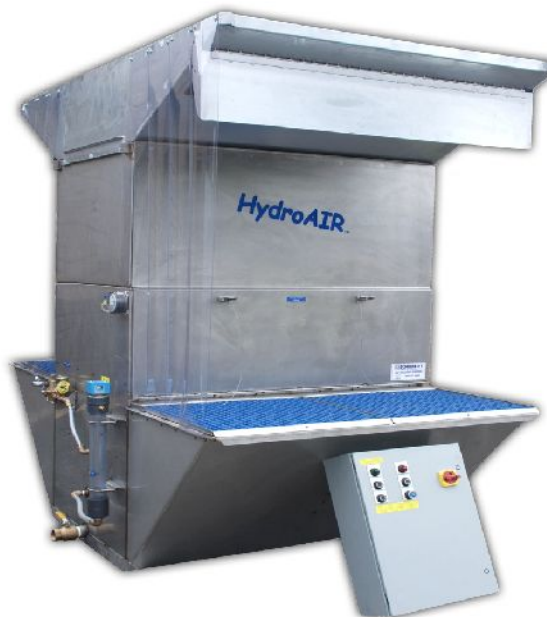
Below: Double Wet Table with Optional Vinyl Strip Curtain Sides and RegainAIR Overhead Canopy. Shown also with Auto Water Level Control and Magnetic Starter Panel.
