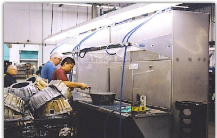
Above: Bank of tables in full production on deburring of aluminum transmission housings. Shown with optional canopy/strip sides.
